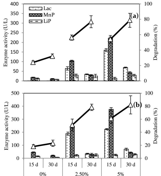
**Figure 5** Comparison of degradation rate and ligninolytic enzymes with rice straw as a co-substrate at pH 4.5, non-saline (a) and pH 8.2, saline
