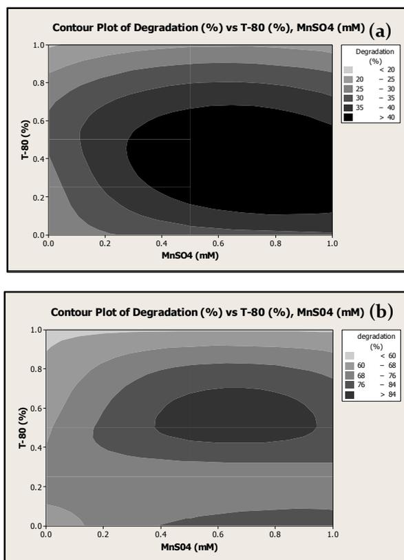
**Figure 1** Contour plot of the biodegradation of BaP versus MnSO<sub>4</sub> and T-80 for 15 days (a) and 30 days (b)
