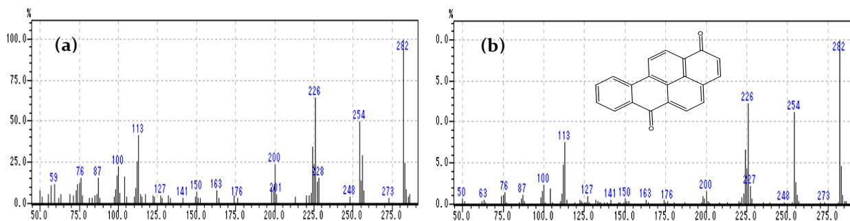
Figure 8 Mass spectra of standard (a) and sample (b) BaP-1,6-dione
