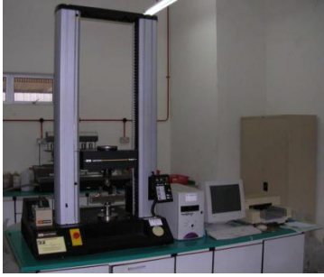
Figure 3 Universal Testing Machine - for tensile and flexural testing
