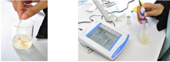
Figure 2 Test the water using pH paper and pH meter AB 15 to determine pH level
